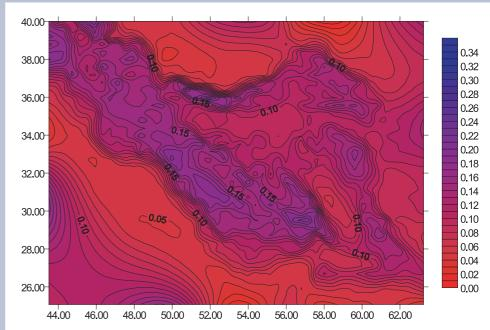
Fig. 3. The direct atmospheric gravity effect with the new formula. Units in mGal.
