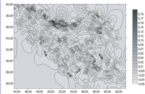
Fig. 4. The differences on direct atmospheric gravity effect between the old and new formulas. Units in mGal.
